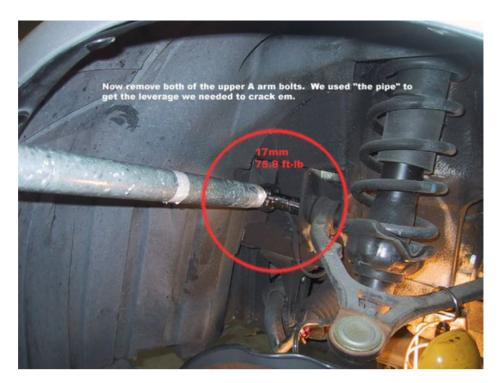
unscrew the top two nuts (note: the torque specs are listed for when you put on the new shock)
