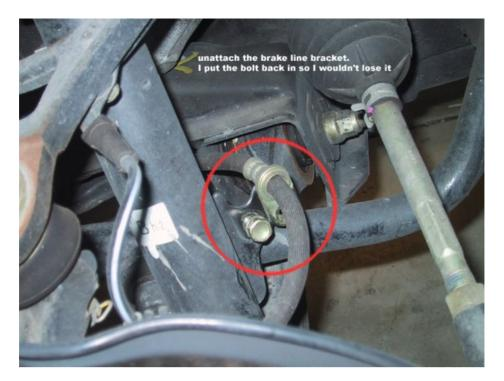
Now unscrew the bolt tot he lower bracket of the shock. (note: the torque specs are listed for when you put on the new shock)
