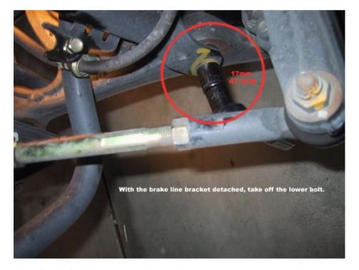
Take off the "A" arm bolts. It should swing forward, just let it rest gently. (note: the torque specs are listed for when you put on the new shock)
